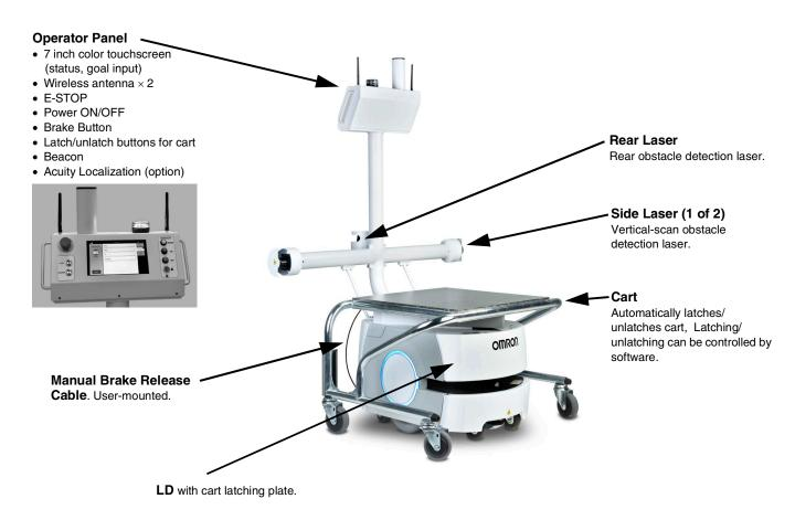
The cart comes with a manual brake release. The user decides where on the cart or its payload structure to mount the manual brake release lever.
